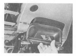
Cut out openings with a piercing saw or metal shears and, if necessary, smooth edges with a wood grater or file.
