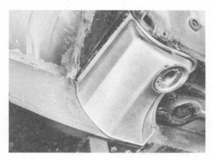
11. Position console for stabilizer on side member (295 mm from front cross member bolt, rear edge vertical) and weld to side member.
