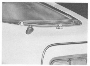
Mount seal on inner frame. Mount bracket on inner frame with M 6 x 16 oval head screw and on spoiler with M 6 x 10 hex. head screw with washer.
