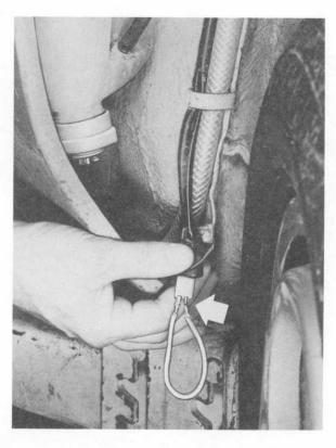
The float switch is located in the right wheel house behind the rear cover.
