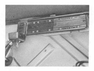
4.1 Installation of the C-Net transceiver unit with accommodation of the excess length of the cable harness.
