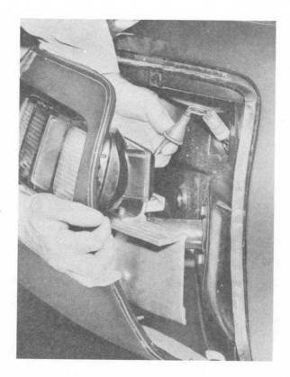
3. Tail lights can be removed with the panel, if rubber grommets are pulled out of tail panel and the then accessible plugs are disconnected.
