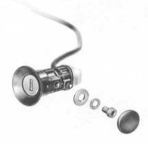
Doors with the new mounting point and new door lock cylinder require a spacer, 6.4 mm dia. washer, and a M  $6 \times 18 \text{ mm}$  fillister head screw.
