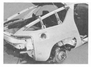
8. Spot weld fender flange all around and weld mating surfaces.
