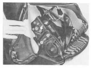
Detach front seat cover and pull up far enough, that motor is accessible from front and can be removed.
