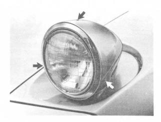
5. Remove 3 small Phillips screws (arrows) from sealed beam securing ring and remove ring.
