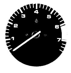
The upshift indicator will light up when it is practical and economical to shift up into the next higher gear. It works in gears 1 through 4 and remains illuminated until the next higher gear is engaged or the operating condition causing illumination of the indicator is changed (e.g. coasting, full throttle, etc.).
