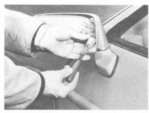
4. Unscrew fillister head screw on mirror base so that mirror can be removed with the liner.
