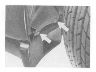
2.Pull front air dam horizontally off mounting clamps.
