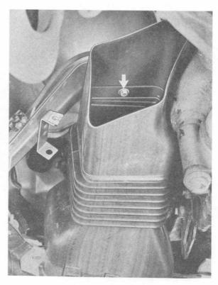
4. Install wheel well cover and secure with washers and 5.5 x 16 mm metal screws. Place and secure spacer behind fender rim. On left side also mount air guide hose on wheel well cover. Secure plug on outside temperature sensor with a hose clamp and connect with the wire harness.
