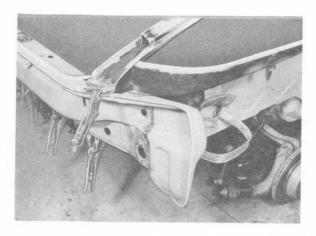
4. Weld both sides of reinforcement bracket on inside of roof frame.
